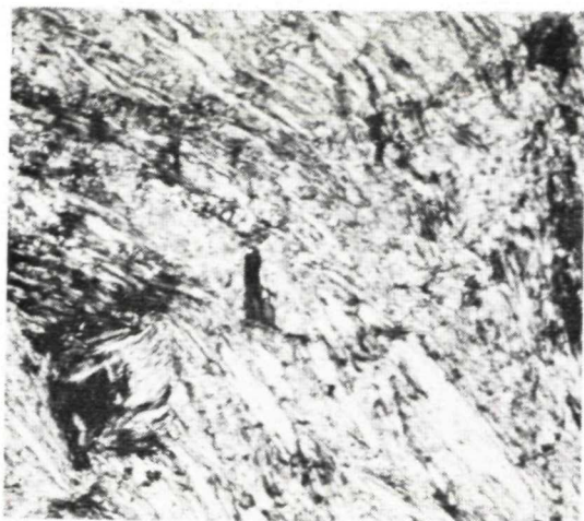
Obr. 2. Usmernenie chloritov v chloriticko-mastencovej bridlici. Sinec, štólna Lýdia, vz. 28, zväčš. 117 \times , skríž. nikoly Fig. 2. Preferred orientation of chlorite in a chlorite-steatite slate. Sinec deposit, Lýdia adit, sample No 28, magn. \times 117 , crossed nicols
